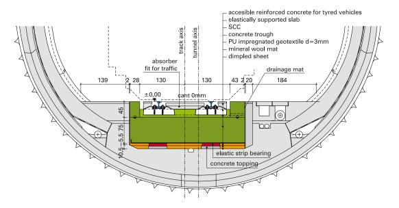
The slab provides a finishing surface with millimetre accuracy. This allows easy and accurate installation without on-site drilling of additional equipment such as noise absorbing slabs, trafficability slabs, buffer stops, track magnets and guard rails.
